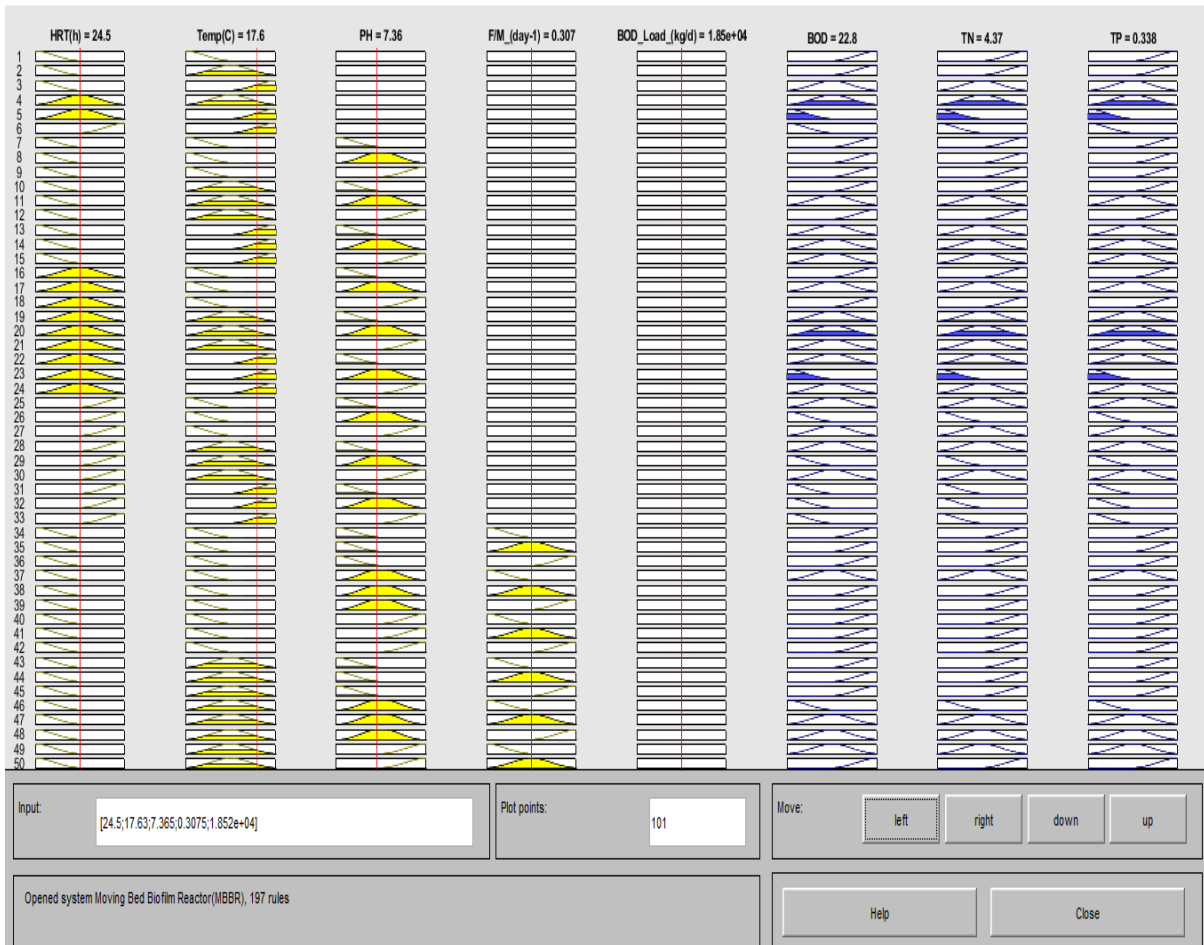
Figure 4. Fuzzy inference diagram for the model predicting effluents the user just needs to put the input values to get the output value as seen from the figure.
