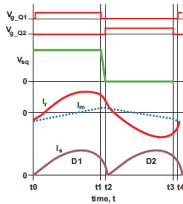
Figure 4. Above resonant frequency
