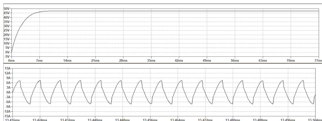
**Figure 7.** Vo and Ir at above resonant frequency
