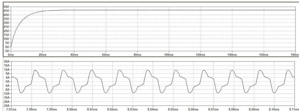
**Figure 6.** Vo and Ir at below resonant frequency
