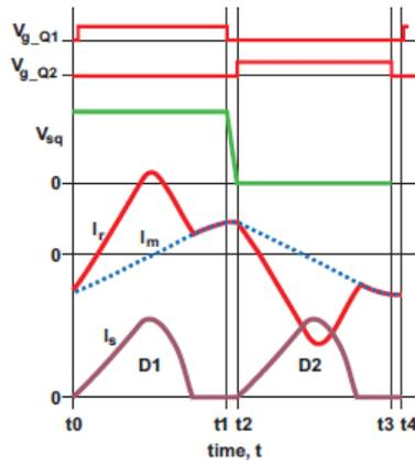
Figure 3. Below resonant frequency
