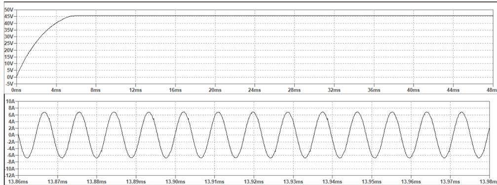
**Figure 5.** Vo and Ir at resonant frequency
