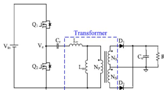
**Figure 1.** Integrated transformer employed for LLC resonant converter
