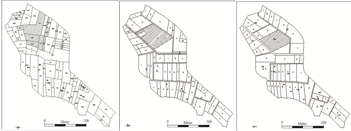
Figure 3. The status of the cadastral parcels (a), its new parcels which occur with interview-based reallocation (b) and its new parcels which occur with block priority-based reallocation (c) belonging to the farmer whose number is 17
